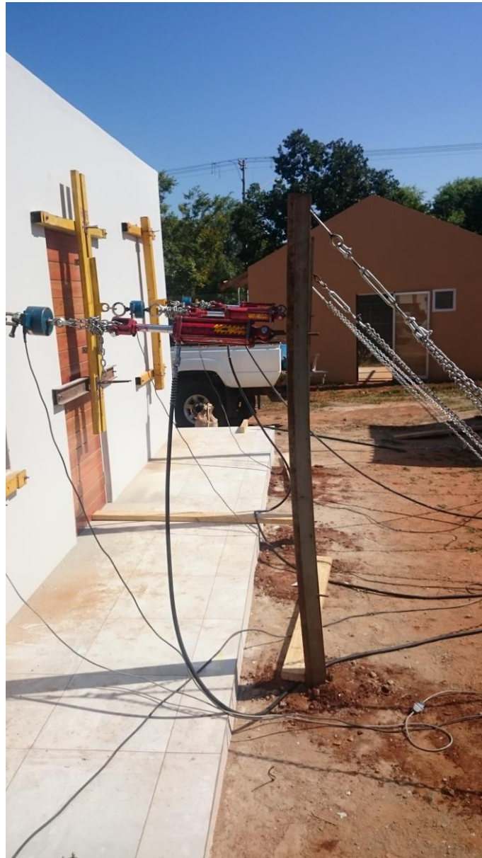
Photograph 1: The test specimen with the wind load brackets attached.
