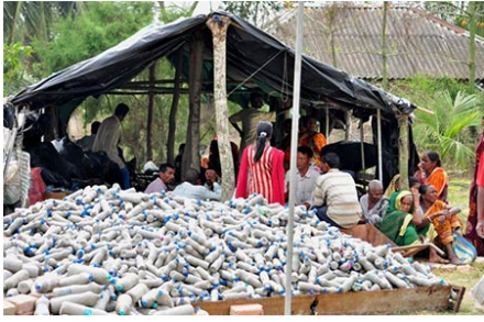
Plastic Bottles filled with mud or sand to be used for construction by Samarpan Foundation
